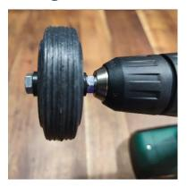
The drill attachment wheel comes with an M8 screw, tightened with a nylon locking nut. Insert the exposed M8 thread into the drill chuck and tighten the chuck **ensure that the attachment is tightly secured in the drill before operating**. A test of the drill will show you if the attachment is installed straight.
