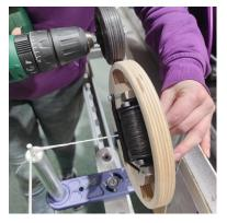
Using the drill attachment wheel, operate the spinner until you reach the desired location.
